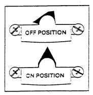
Selective Click: If you would like to remove the clicking sound, this can easily be accomplished simply by removing the spool and positioning the triangular click pawl in the off position as illustrated. In this position, your drag will remain operational, but there will be no clicking sound when the spool is revolving either forward or backward.
